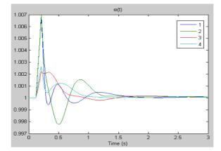
Figure 10: Rotor Speed Variation  $\boldsymbol{\varOmega}$  after Optimization
