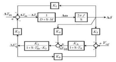
Figure 3: Linearized Model of SMIB System
