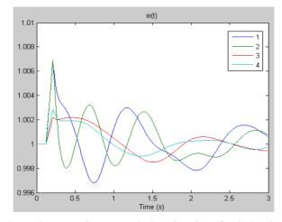
Figure 9: Rotor Speed Variation  $\boldsymbol{\varOmega}$  before Optimization
