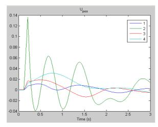
Figure 7: Power System Stability Constant  $U_{\text{PSS}}$  before Optimization
